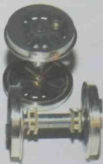
Left Painted wheelsets ready to go back into the chassis. Even though these come in a black finish, the etched metal counterweights provided in the kit need to be painted. Note the spacing washers on the axle to control side play, and those shiny wheel treads. The brown ring visible on the wheelset at the back is rim insulation.
