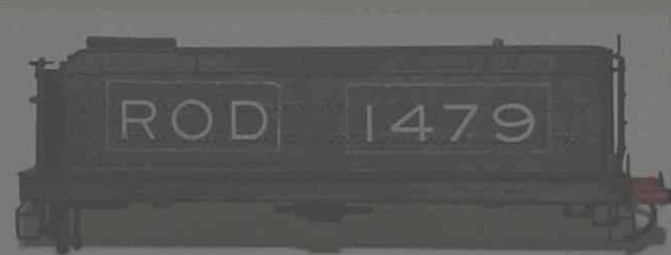
Above Transfers on the tender after application of decal film softening solution. Note the white 'bleed' where the solution has crept under the cut edge of the transfer film and dissolved the ink.
