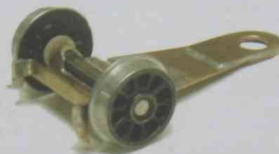
Left The pony truck needed to have its pivot point moved 1mm further forward to bring the front back to be level with the front of the buffer beam.
