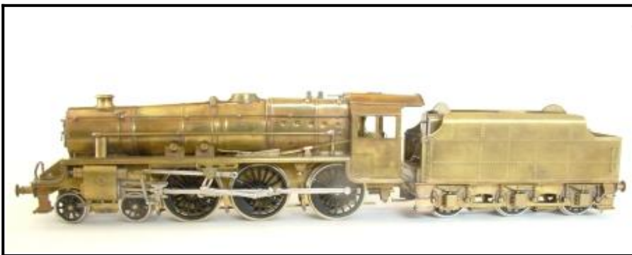
Britrail Black 5 as converted to 18mm EM gauge and awaiting painting
