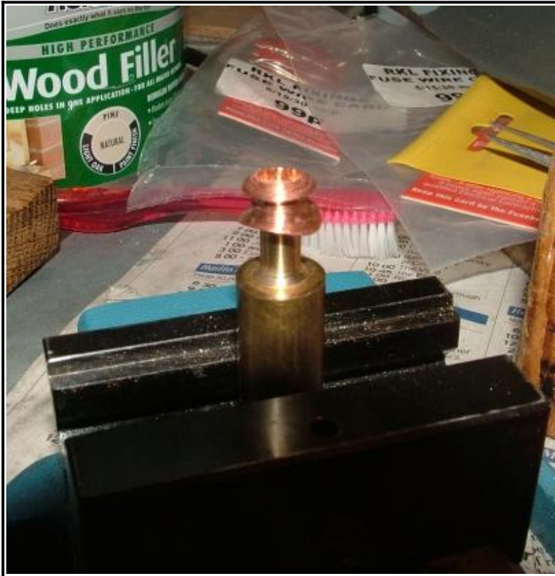
Chimney on mandrel held in 'V' notch of machine vice for shaping of smokebox flange skirt with needle files.
