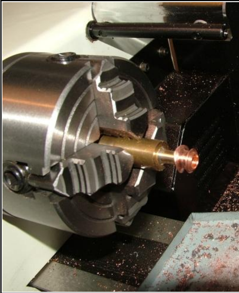
Getting ahead of ourselves here: chimney on push fit brass mandrel set up for polishing of cap.
