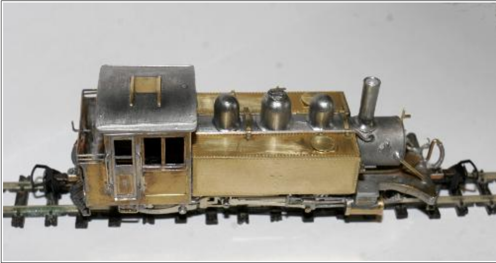
Top view - RH blower pipe clipped to top of tank stays.
