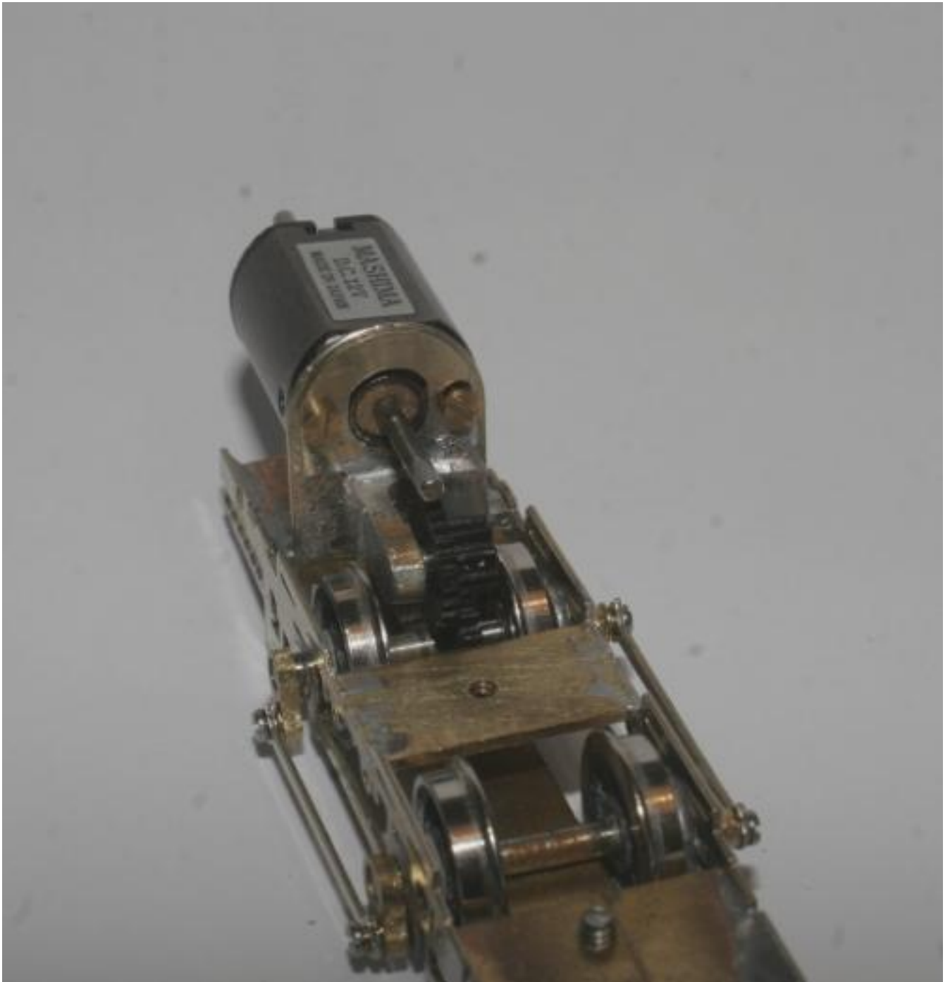
Motor mounting showing intermediate idler gear 'outrigger' shaft.
