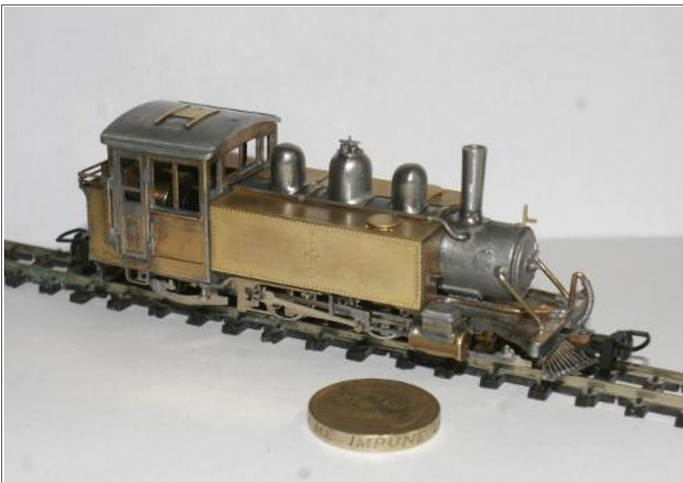
Could not resist this one - the pound coin gives you an idea of the size of the completed locomotive. Front lamp iron is filed and sawn from 1mm brass plate - far stronger than folding it from strip or etch.
