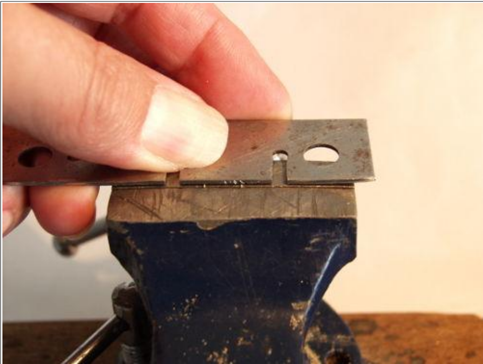
Making drop grab handles 2. Then carefully bend the upright handle flat, using a metal plate that is wide enough for leverage.
