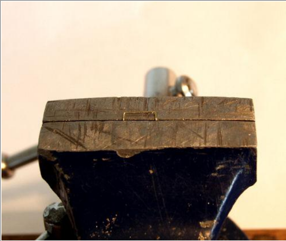
Making drop grab handles 3. The finished grab handle.
