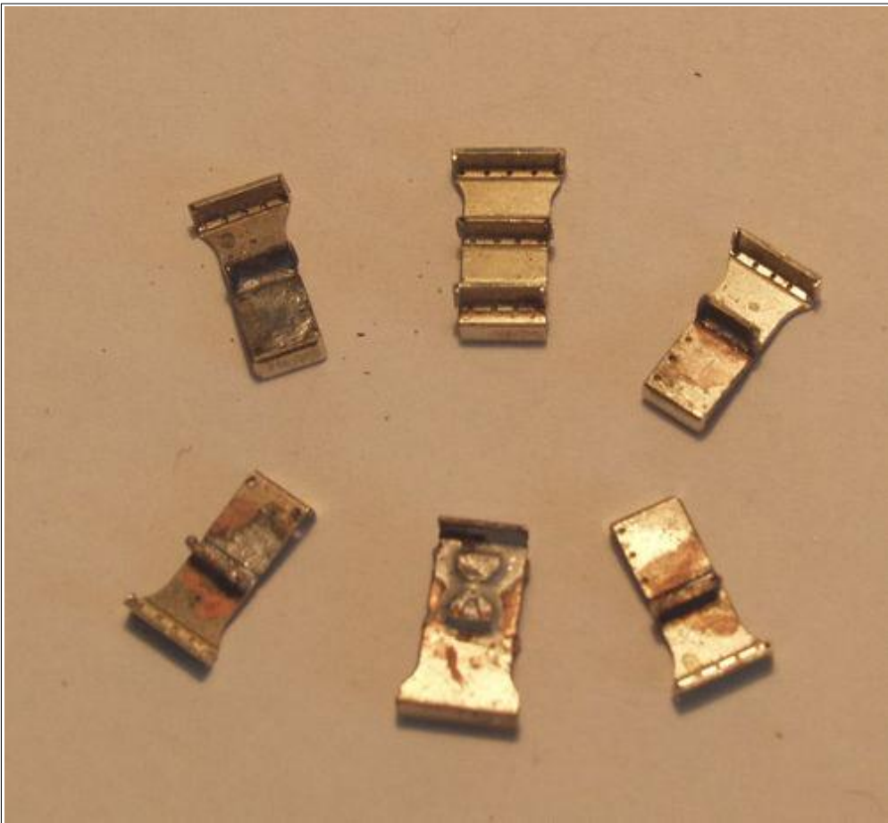
Cruel enlargement of the six footsteps. Beware - the two wider of the six have three treads and go under the cab, and yes, first time around I got the in the wrong place. Soldering these up was a bit more fraught than usual, in that I had to clamp the middle tread set in place with a pair of forceps, before moving on to the top one, This is where you need a hot iron, despite the small size of the component, to stop the heat leaking away into the clamp.
