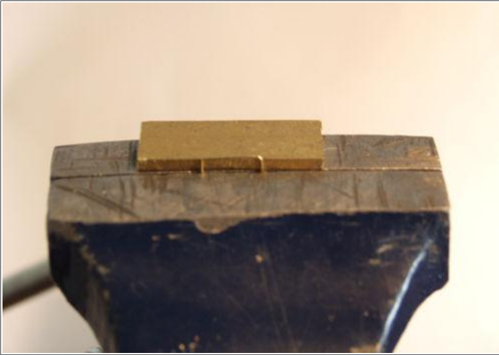
Making drop grab handles 1. The handle is bent up in the usual U, and then set end on in a vice so that it is level with a scrap piece of bar the same scale height as the finished handle.
