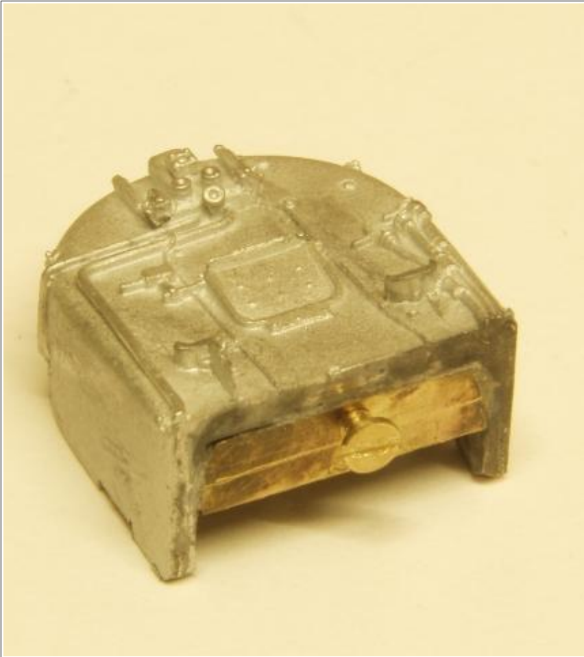
Backhead with soldered on tapped bracket for secure fitting inside cab.
