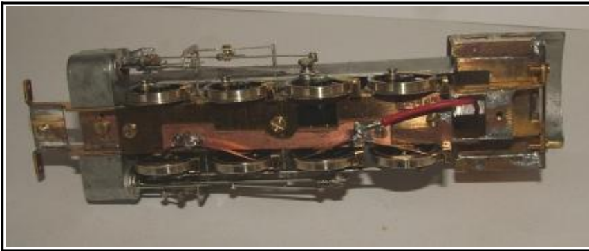
Electrical current collectors on loco. Note the brass slotted 'pegs' in the copper clad paxolin that hold the phosphor bronze strip wipers.
