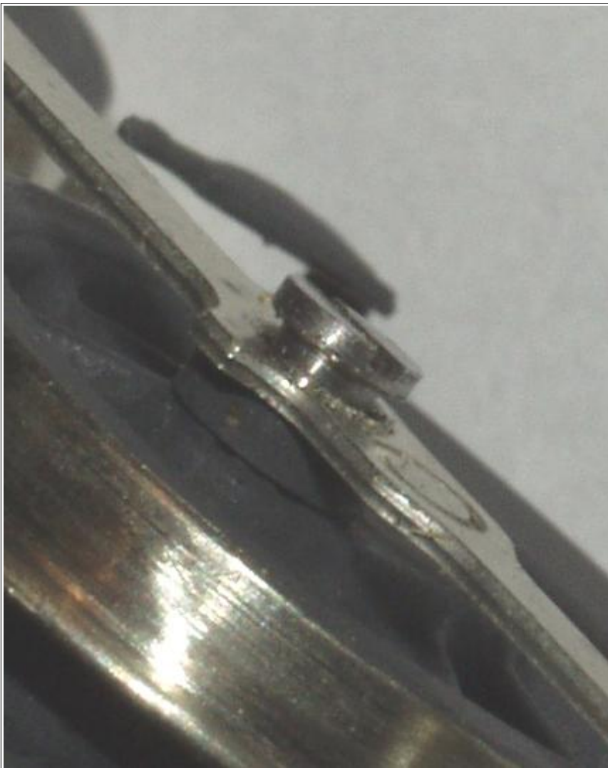
Cruel enlargement of crankpin screw on second driving axle, left side. Look carefully and you can just make out that the screw head is tilted out of parallel with the wheel - and it was this that was causing the coupling rod to bind on that side. Black 'crescent' shape to top of picture is etched brake shoe.
