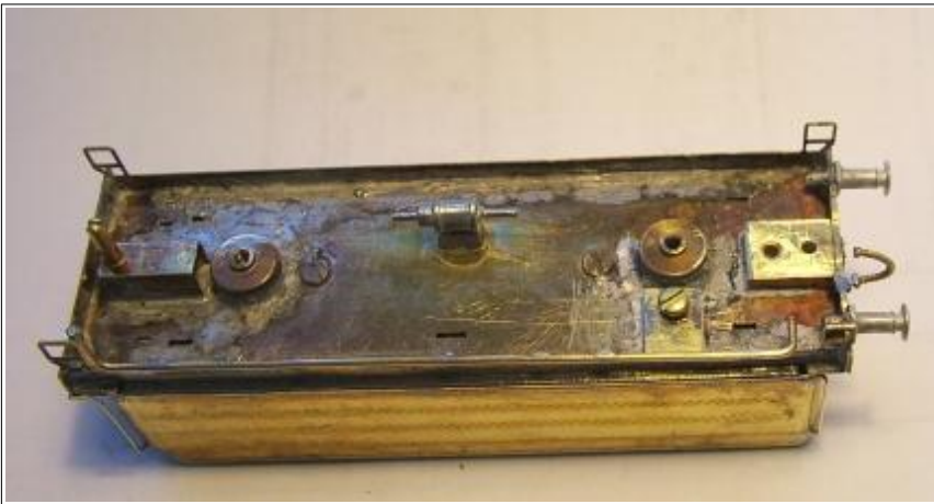
Tender inverted. Note the Kadee coupling mounting pad, and the adjusting screw - secured with Loctite - to set the tender level and prevent the rear truck (bogie in Anglo-Saxon parlance...) from wobbling around its central pivot.
