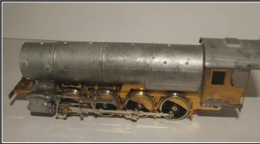
Chassis assembled with Walschaerts gear and checked for free rolling on the level..
