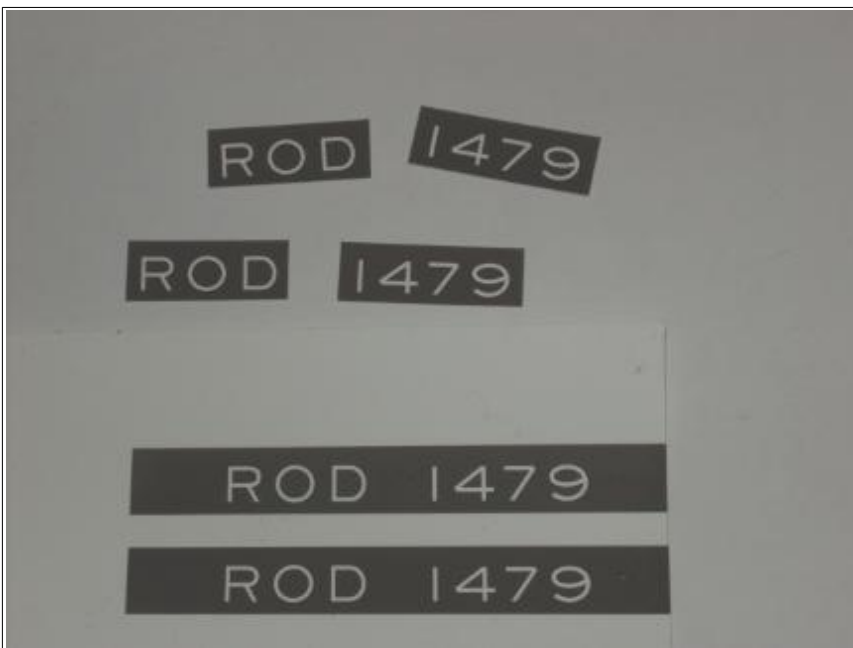
Transfers were made on an inkjet printer, then sealed with acrylic matt spray - this does not affect the inks, and seals the transfer from water during the separation of carrier film and paper backing.
